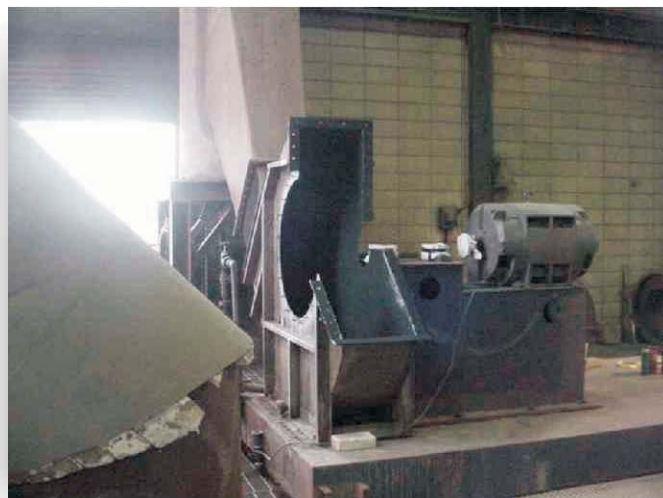
Two coats of CHEMCLAD XC were applied to all interior surfaces and flanges.
