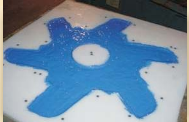
A special mold was created to allow consistent thickness of the trowel applied DuraTough DP.
