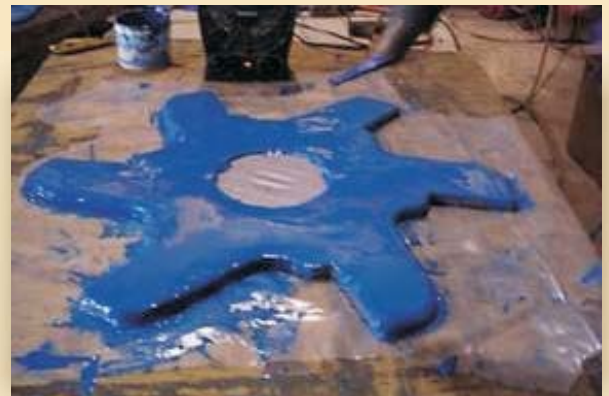
The wear plate after the application of DuraTough DL with the mold removed.
