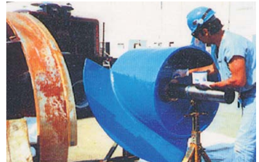
Putting the finishing touches on the impeller.
