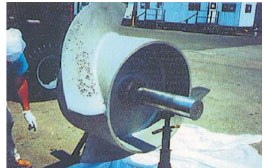
The pump impeller, after grit blasting.
