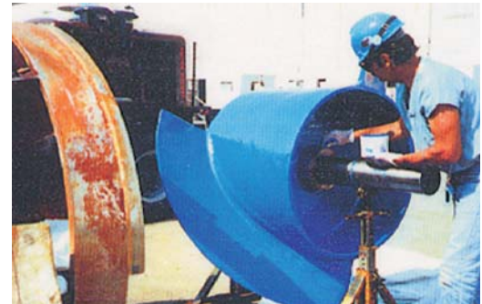
Putting the finishing touches on the impeller.
