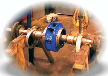
The pump impeller and bottom casing after 9 months continuous duty, showing the DuraTough DL protection of the impeller surface is still in good condition.
