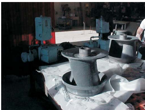
CeramAlloy CL + AC was used to treat any areas not covered by CP + AC
