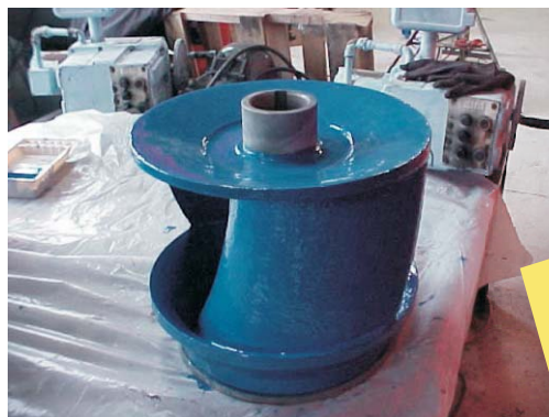
Finished impeller after second coat of CeramAlloy CL + AC
