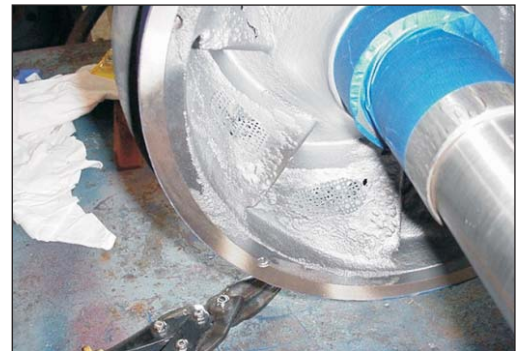
Reinforcing 'mesh' and DurAlloy applied over holes
