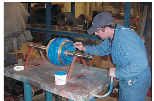
CeramaAlloy CL+AC being applied
