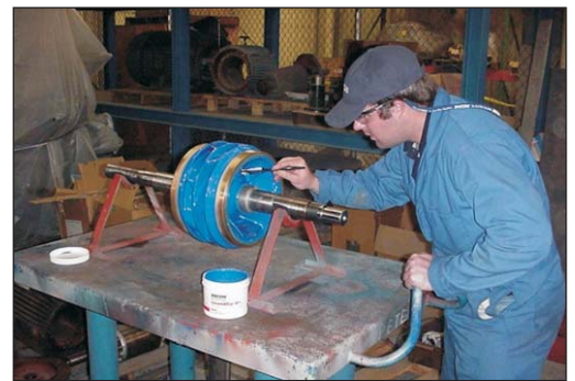
CeramAlloy CL+AC being applied
