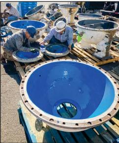
When it comes to superior protection of its most critical components, the U.S. Navy routinely turns to ENECON and specifies *METALCLAD CeramAlloy CL+AC* to repair and protect its fluid flow components from erosion & corrosion damage from sea water.
