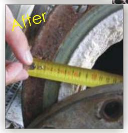
The maintenance engineers at this large power station - one of the biggest - in Poland had been experiencing a verv severe mineral (lime) scale problem in their cooling water lines which carry water from a nearby lake. This scaling was so severe that it often rendered the pipes "useless" necessitating extensive cleaning or replacement.
