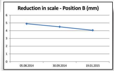
Scale measurements at 2 different positions show reductions in scale over time.
