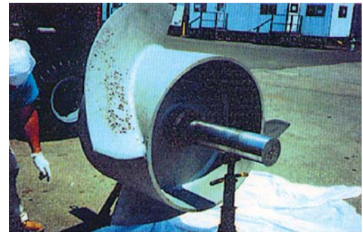
The pump impeller, after grit blasting.
