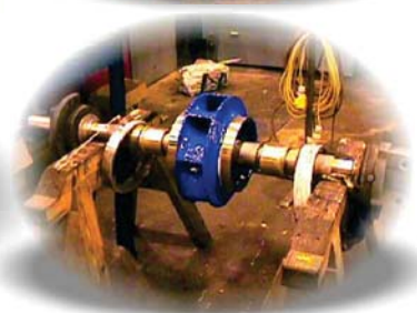
The pump impeller and bottom casing after 9 months continuous duty, showing the DuraTough DL protection of the impeller surface is still in good condition.
