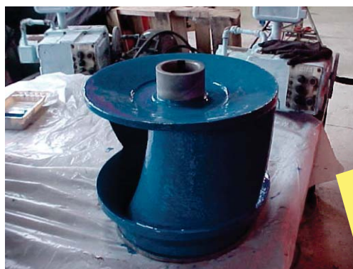
Finished impeller after second coat of CeramAlloy CL + AC
