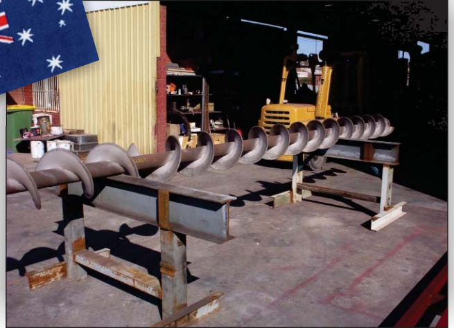
Conveyor after grit blasting
