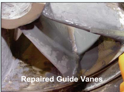
Expanded Metal Mesh Used to Reinforce Damaged Guide Vanes
