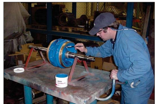
CeramaAlloy CL+AC being applied
