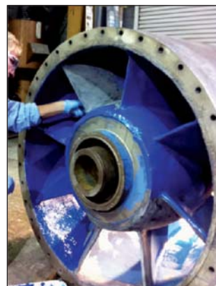
CeramAlloy CL+AC used to coat all surfaces.
