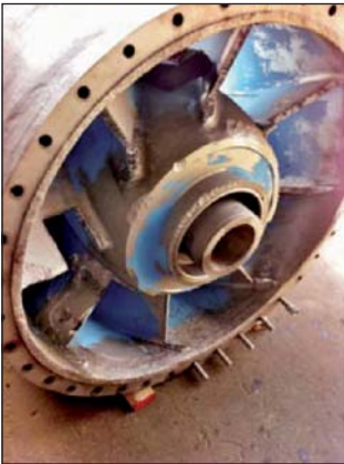
The severely eroded vanes were cut away.
